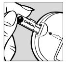
1 Insert the Check Strip fully into the Meter as shown. NOTE: If your Check Strip is not available, you can use a **new** Test Strip for this procedure. However, you have to wait 3 minutes for the memory sequence to begin.
